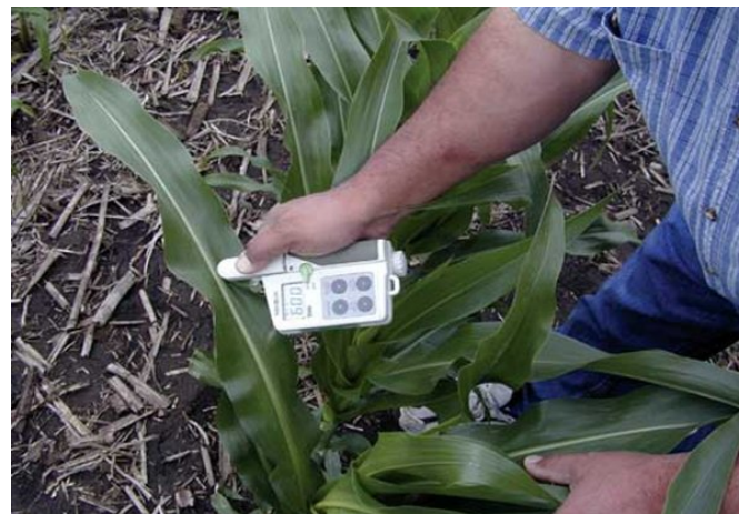
Figure 3. A chlorophyll meter is used to collect readings in corn. Source: John Sawyer, Iowa State University.
