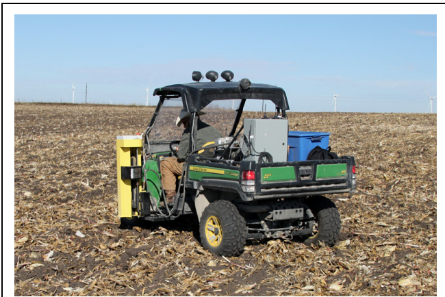
Figure 2. Soil sampling a large field with a mounted hydraulic sampler.
