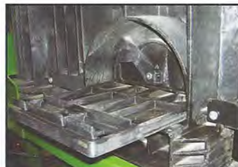
Seed Box Slide Gate allows for changing Seed Varieties on the Fly
