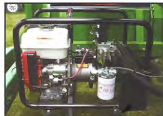
Honda™ OHV Electric-Start Gas Engine - Self-Contained Hydraulic System
